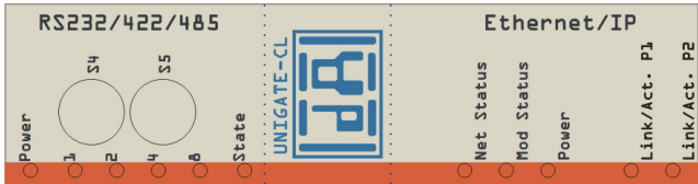
Picture 2: Front panel: Rotary switches, LEDs
