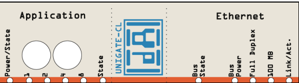
Bild 2: Front panel: Rotary switches and LEDs
