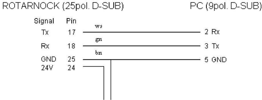
A voltage supply to the pins 24 (24V) and 25 (Gnd) has to be made externally.
