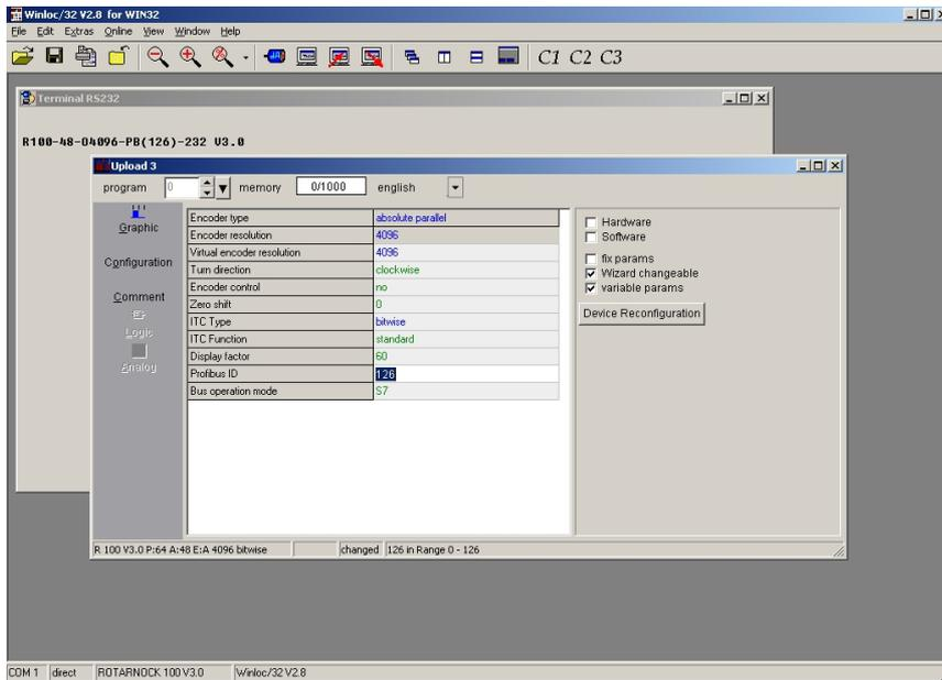
A „Download“ has to be performed in order to take over the change. The device carries out a restart and with it the new ID is set.
