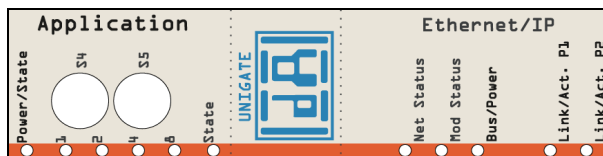
Picture 2: Front panel: Rotary switches and LEDs
