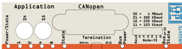
Picture 2: Front panel: Rotary switches, LEDs and termination CO
