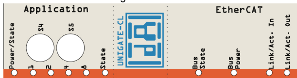
Picture 2: Front panel: Rotary switches an LEDs
