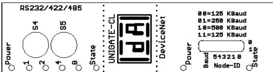
Picture 2: Front panel: Rotary switches, DIP-switch and LEDs
