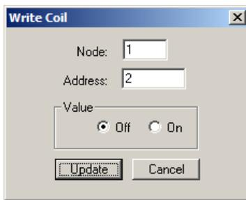
Address 0002 stays unchanged on 0, however, the fieldbus output data is updated.
