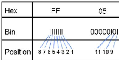
Please keep in mind that No. Of coils = 10, hence, only the lower bit in address 0011 is written at the value 0x05. Address 0013 would already be bit No. 11, which is not transmitted anymore.
