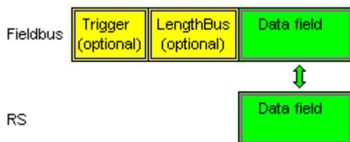
On the RS-entry side the timeout time of 2 ms is firmly set. If no more data is received within the timeout period, then the data that has been received so far is transferred to the bus.
